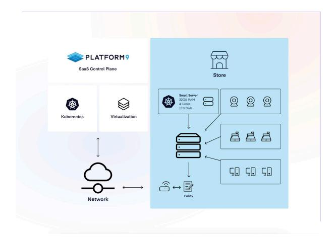
Each store connects to the main-office network via an in-store WAN router to the VPN internet connection and then to a managed Kubernetes instance at their headquarters. Each location typically includes a router with different networking policies, CCTV and POS/IoT devices, and customer access to the hotspot.
